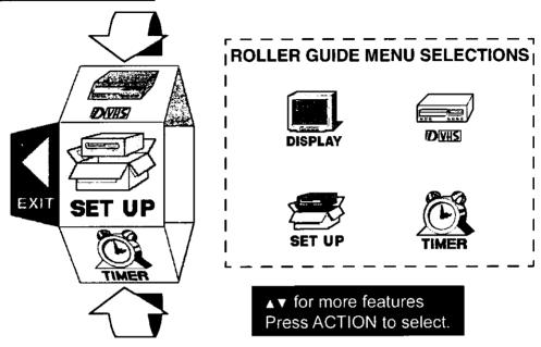
Note: To exit the Roller Guide Menu, press the ☐ arrow on the ACTION button or press the MENU button.
